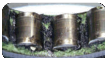
Initial Arcing causing High temperature Stress of Grease
