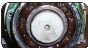
Hardening of Grease, stops Relubrication
