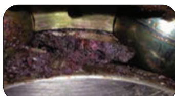
Oil destroyed in grease, only Polymer remains
