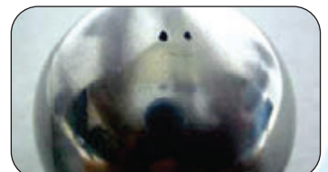
Light brown marks and pitting
